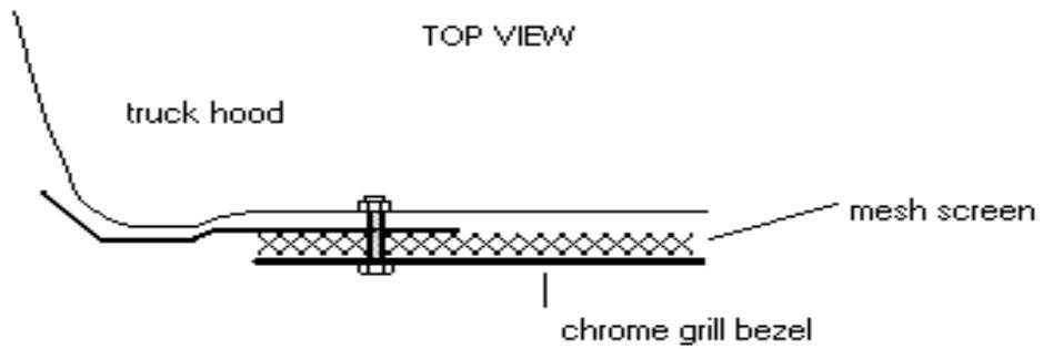
3. Slide the bolted hole flange in behind the mesh screen and chrome grill bezel. The Grill Deflector hole flange should be against paint. (see diagram above)
