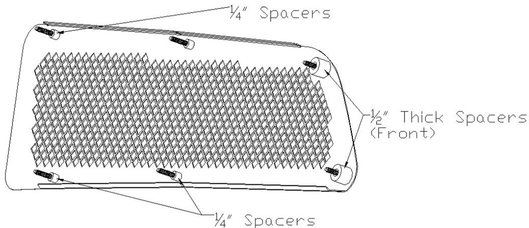
**NOTE:** As a helpful installation tip, the spacers can be secured to the grille intake with silicone and left to cure prior to install. Tape can also be used to secure the spacers.
