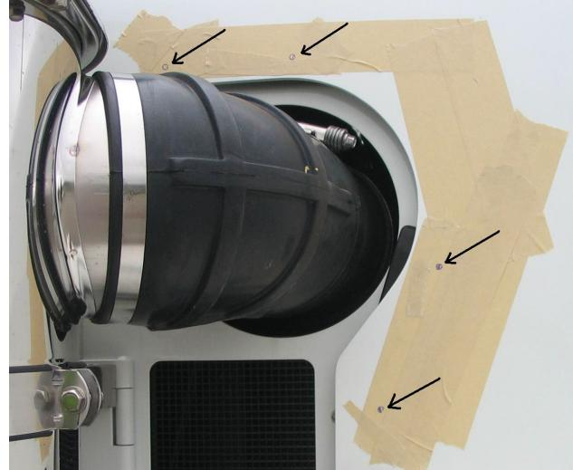
**IMPORTANT: Prior to drilling any of these holes, please check for clearance around the reinforcement of the hood. The hood has a reinforcement rib on the inside at the location shown →**
