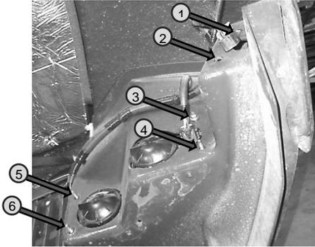
Figure 4 Headlight/Signal Nuts
