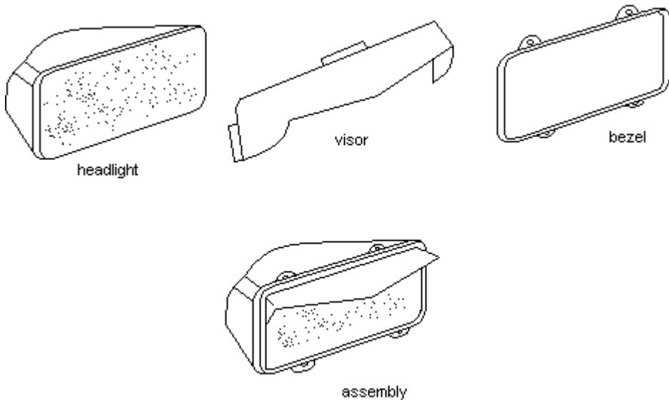
3. Loosen the stainless steel retaining ring enough to facilitate the clamping of the visor tab between the headlight, and retaining ring. (see diagram above)
