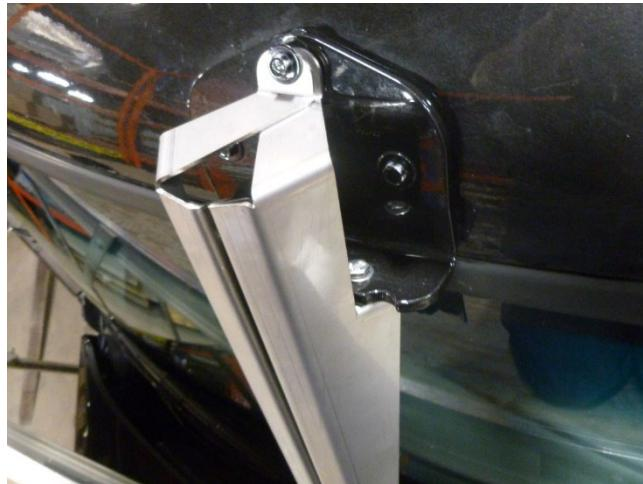
5. Set the visor halves on the truck with the horizontal flange of MBDU/MBPU under the corresponding OEM brackets
