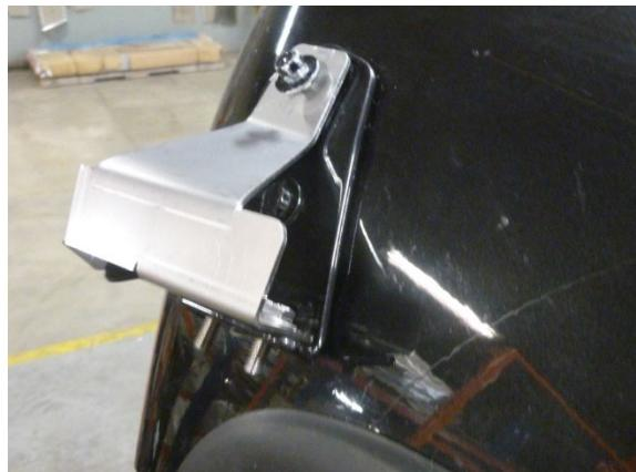
4. Mount the Center Brackets loosely in place, with the passenger bracket on top of the driver bracket, and both brackets under the OEM bracket (see photo below)
