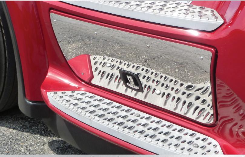
High quality 304 stainless steel kick panels. Fasten using supplied hardware, drilling required. Designed for 2013+ Peterbilt 579 models with chassis fairings. Available as a set or individually.
