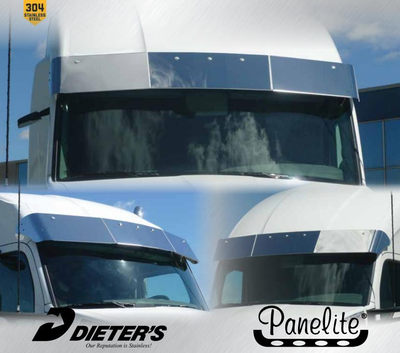
Designed for Kenworth T680 and T880 Mid-Roof and High-Roof sleepers. For models without an existing sunvisor. There are 10" and 12" drop options - both sizes available with either 5 or 9 3/4" round LED lites. Brackets, hardware, lites and harnesses included.
