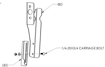
FIGURE 3 – Inner bracket sub-assembly, driver side shown
