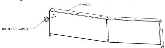
FIGURE 5 - Center Wire Cover, grommet installation
