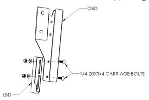
FIGURE 2 – Outer bracket sub-assembly, driver side shown
