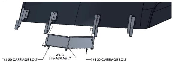
FIGURE 8 - Center Wire Cover, shown from front view
