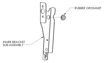
FIGURE 4 - Inner bracket sub-assembly, driver side shown
