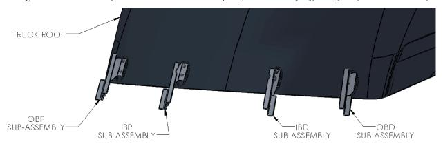
FIGURE 7 - Brackets mounted to truck, shown from front view
