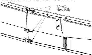
FIGURE 11 - Center bolts, shown from rear view
