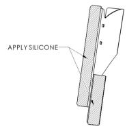
FIGURE 10 - Bracket sub-assembly, silicone application, shown from front view
