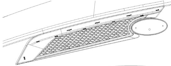
2. Put masking tape on the back edge of the bracket and roughly place the bracket. There are three holes for OE grille to hook onto. Mounting holes on bracket should not be on the same spot.
