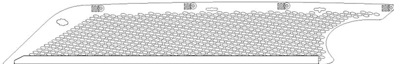
7. Install the bracket and dry fit the grille. Adjust the bracket so rear part of the grille aligns with truck contour. The truck has curve so either end of grille cannot be mounted flush. Front end will be covered with bezel, focus on middle and rear end.
