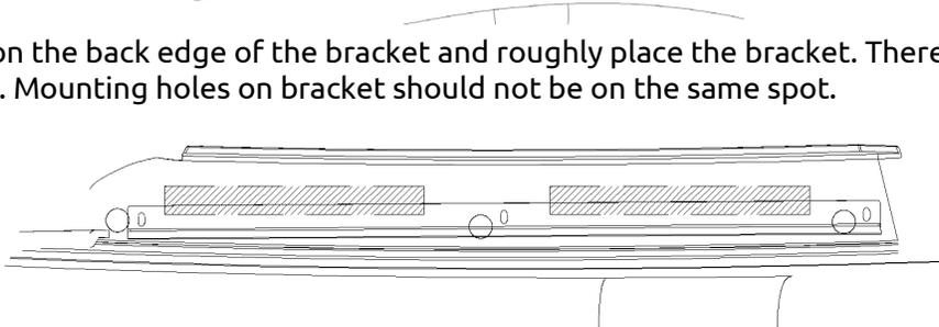
3. Place the grill and push the bracket inwards. Masking tape should keep the bracket in place.
