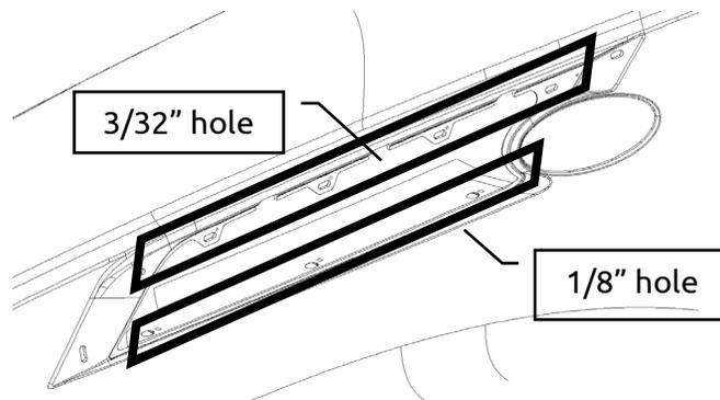
6. Tape the nylon spacers behind the mounting holes of the grille to prevent from falling while installation.
