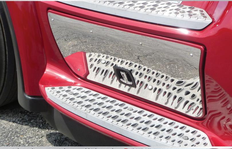
High quality 304 stainless steel kick panels. Fasten using supplied hardware, drilling required. Designed for 2013+ Peterbilt 579 models with chassis fairings. Will not fit New Model/MLU 579. Available as a set or individually.
