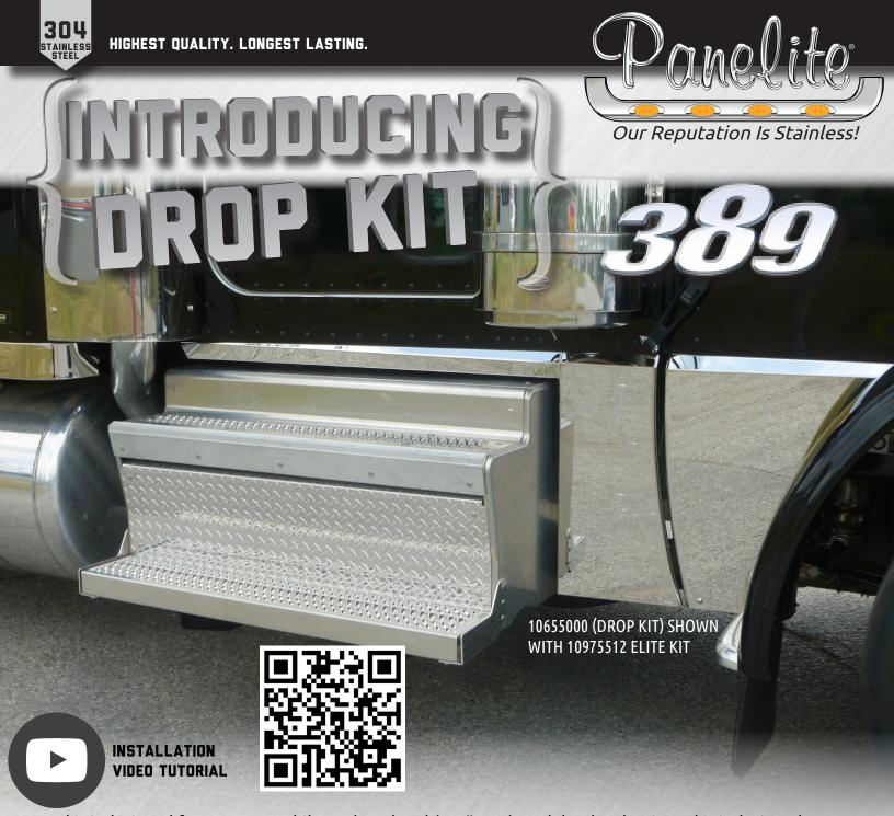
Drop kit is designed for 2018+ Peterbilt 389 long hood (131" BBC) models. The aluminum kit is designed to replace the OEM piece and lowers the DPF box 1.5" to allow for more room between the top step and the cab. Sold individually.
