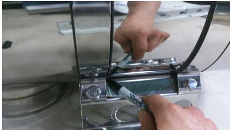
3. Remove the factory bracket and straps. The polished bolts will be re-used to attach the new assembly to the truck.
