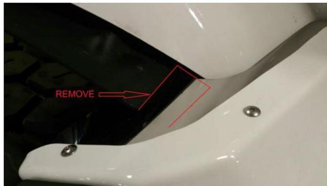
3. Remove two of the bolts shown below to allow easier installation of the splash shield.
