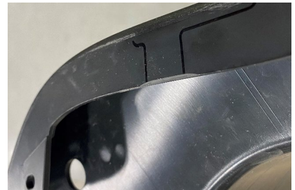
Fig 2: Chamfer Needed for OEM Mid Roof Panels
