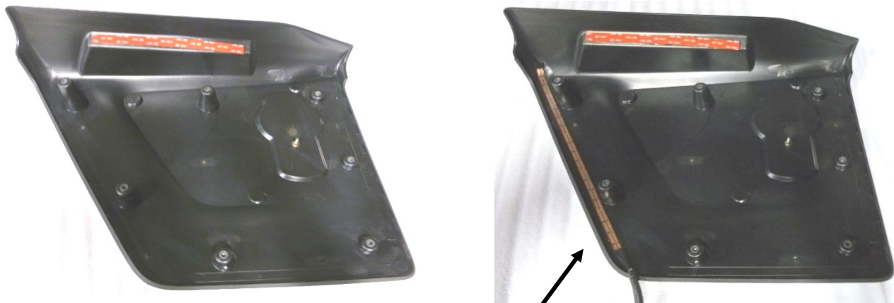
Intake Accent Light strip install
