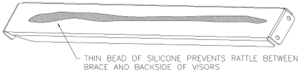
Fig. 2: Applying Silicone to the Support Braces
