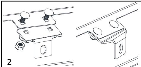
3. Install rear mounting bracket to the cab using the supplied 1/4-20 X 1/2" hex head bolt, 1/4" lock washer.
