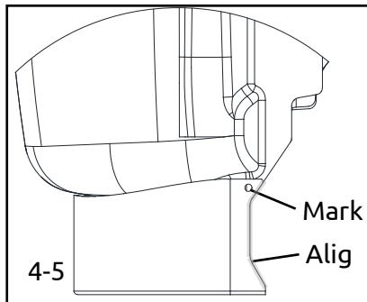
6. Install cab skirt on the truck with supplied 1/4-20 X 3/4" hex head bolts, flat washers, and lock nuts on the locations marked in the image below. Do not fully fasten.
