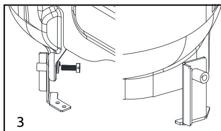
4. Hold the cab skirt aligning the rear contour of the cab skirt to the truck and mark the location of mounting hole
