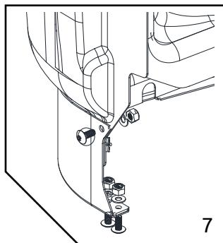
8. Fully tighten the front mounting bracket to the cab, and then the cab skirt to the mounting bracket. Control the gap between the skirt and the cap while tightening.
