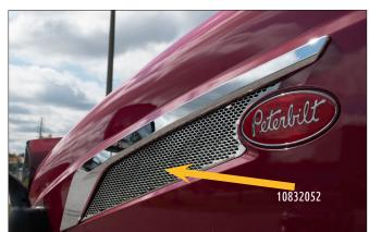
**INTAKE GRILLE** Replaces existing OEM air intake grille with a high-quality 304 stainless steel version. Attaches using hardware and supplied 3M two-sided tape. Sold in pairs.
