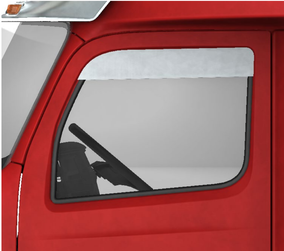
Fig 1: Door Top Cap Installed (579 Shown)
